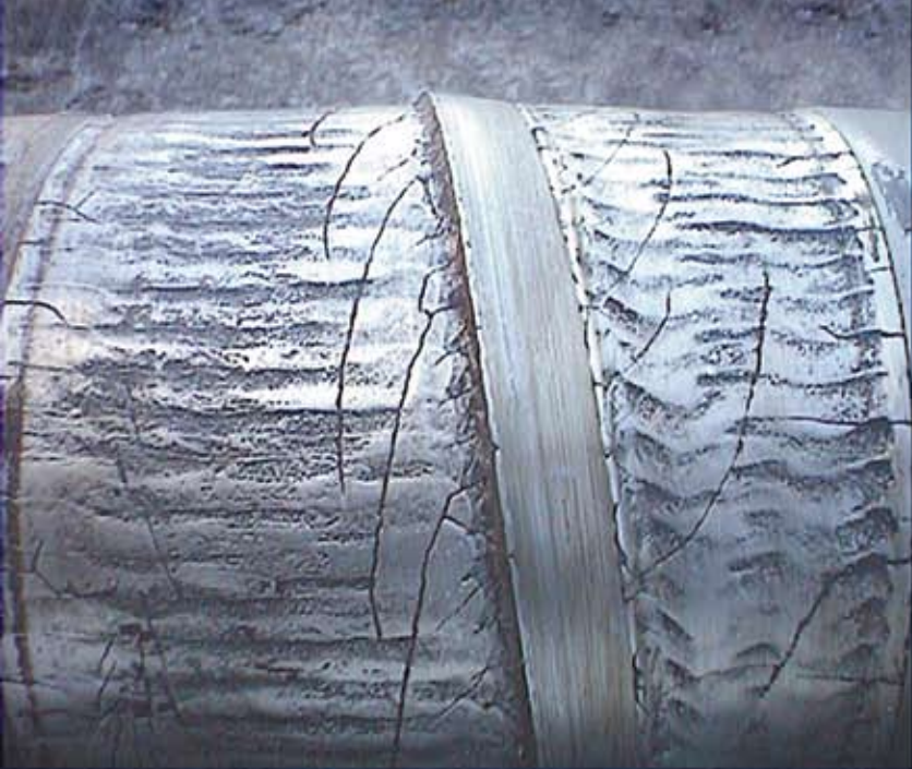
An ordinary screw press shaft flight after 1,940 operating hours.
