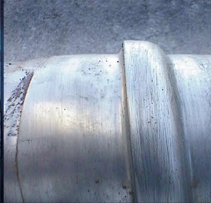
A Dupps Tuff-Cast™ flight after 1,940 operating hours.
